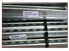
Trapezes and Assemblies can be labeled to correspond with specific locations on drawings.
