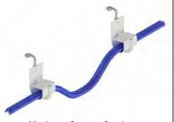
Maximum Support Spacing Illustration for Data Cables
